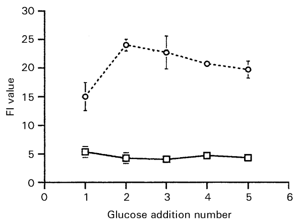
Figure 4. The magnitude of the glucose response upon repeated glucose triggering of a covalently modified glycogen-lectin gel system (○) compared with a dextran-lectin gel system (□).
